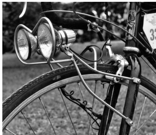
Lighting solutions included this custom-made front rack that carried two generator-powered headlights, but no bag.
