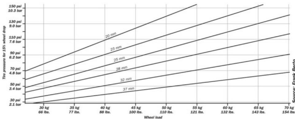
Tire inflation for 15% wheel drop in relation to wheel load and actual tire width.<sup>4</sup> Example: Rider and bike weight: 100 kg. Weight distribution: 45%/55%. Wheel loads: 45 kg/55 kg. Tire pressures for 20 mm tires: 125 psi/155 psi. Tire pressures for 37 mm tires: 45 psi/53 psi. For heavy riders/bikes, narrow tires require very high inflation pressures, and wide tires are a better choice.
